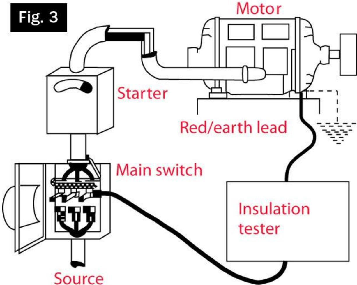
This is the simplest of the tests. After the required connections are made, you apply the test voltage for a period of one min. (The one-min interval is an industry practice that allows everyone to take the reading at the same time. In this way, comparison of readings will be of value because, although taken by different people, the test methods are consistent.) During this interval, the resistance should drop or remain relatively steady.
